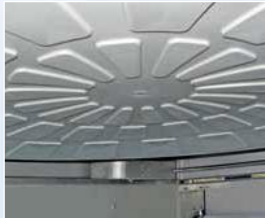
Freely rotating press die for longer membrane lifetime
