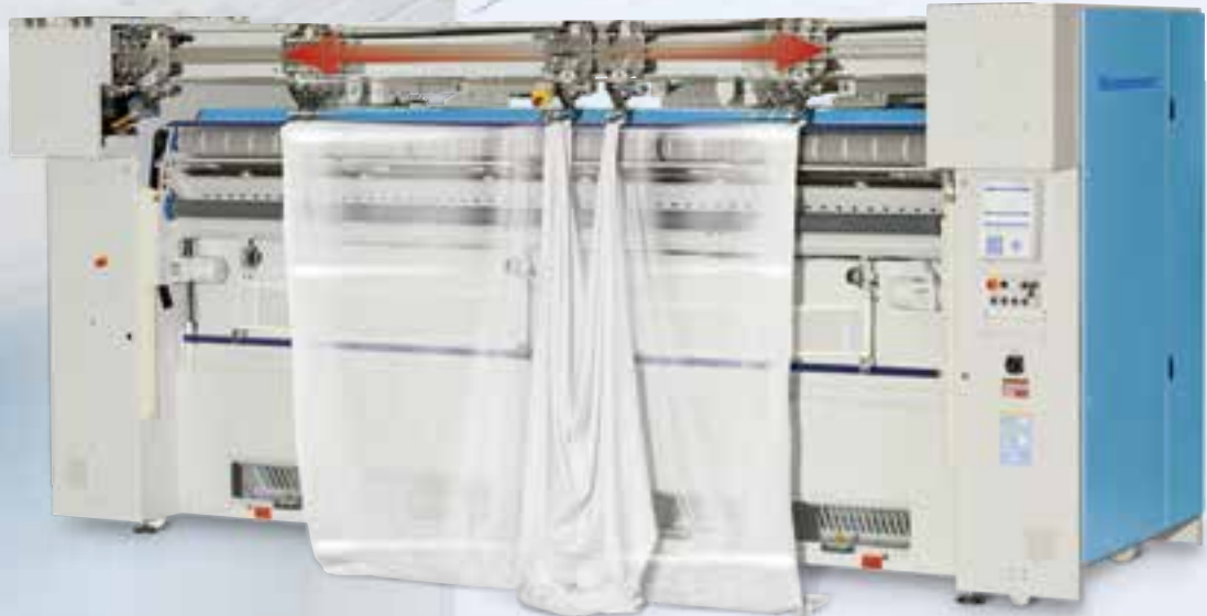
Synchro clamp with large surface clamping area
