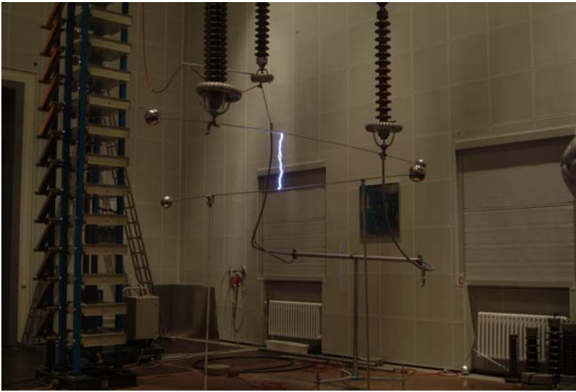
Figure 8: Photographical evaluation „HVI – Light“, wet – tap water
