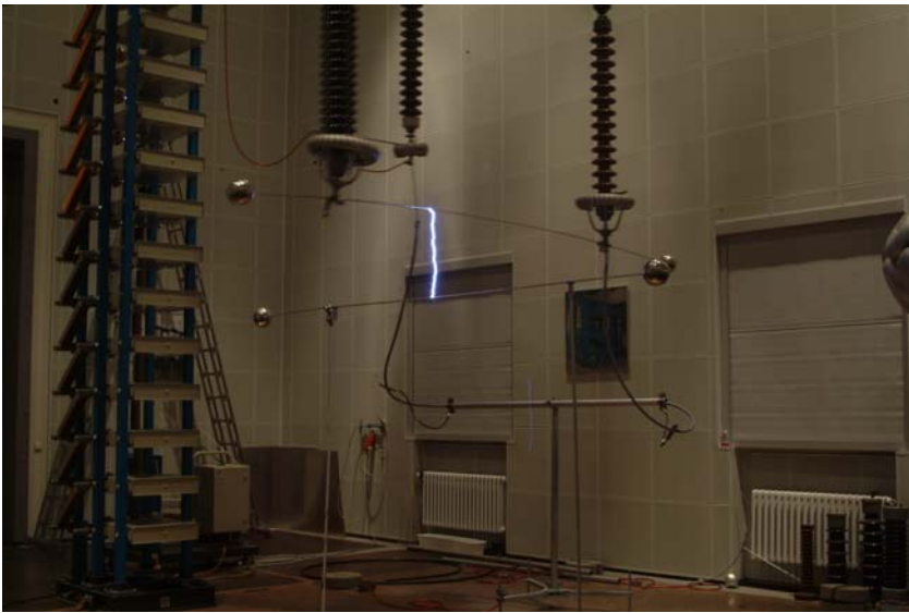
Figure 9: Photographical evaluation “HVI – Light“, wet – 5% NaCl-Solution
