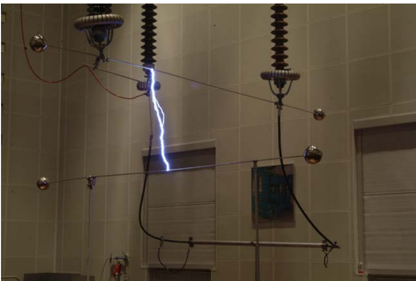
Figure 6: Photographical evaluation “HVI Standard“, wet – 5% NaCl-Solution
